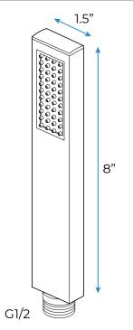
Flow Rate: 2.0 GPM / 7.6 LPM
